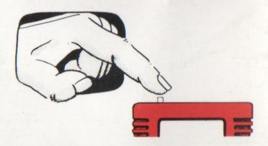
On the back of the POWER CARTRIDGE there is a Reset Button. Pressing this button makes a SPECIAL MENU appear on the screen.
